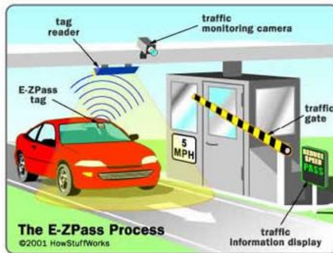
Figure iv - Diagram Showing RFID in action with E-ZPass System
